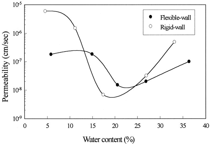
Fig. 7. Hydraulic conductivity vs. molding water content for rigid-wall and flexible-wall cells.
