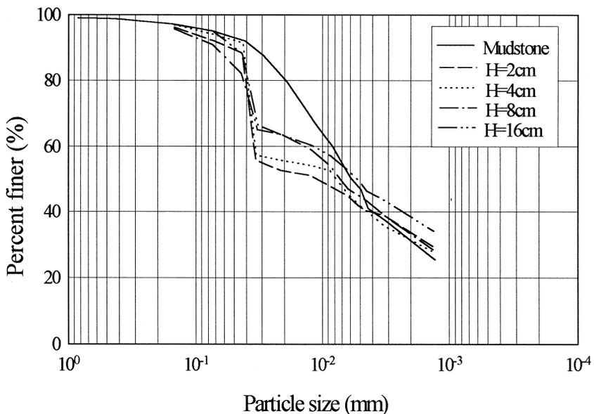
Fig. 4. Particle-size distribution curves of raw mudstone and the permeated mudstones obtained from four different thick liners, respectively.
