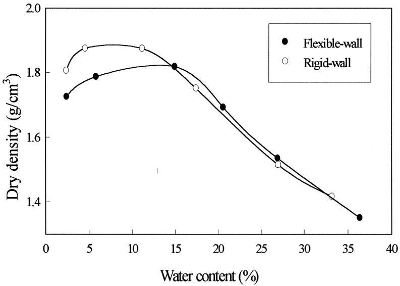
Fig. 6. Standard proctor compaction curves for both rigid-wall and flexible-wall cells.
