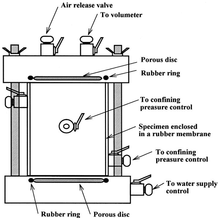
Fig. 3. Rigid-wall and flexible-wall cells used for permeability tests.
