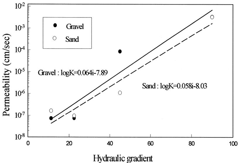
Fig. 5. Hydraulic conductivity vs. hydraulic gradient for mudstone permeated with water using rigid-wall and flexible-wall permeameters.
