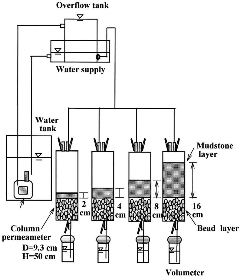
Fig. 2. Apparatus for the simulated column tests.
